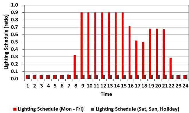
Figure 6. Lighting schedules used for the office-building model.
