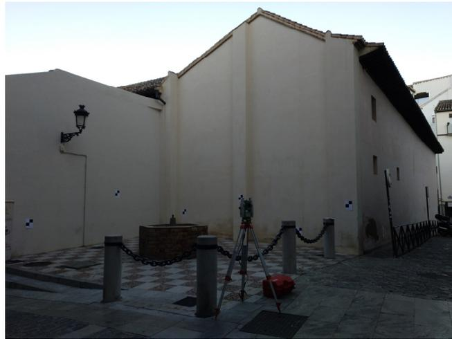
**Figure 9.** Targets for checking the registration of the point cloud.
