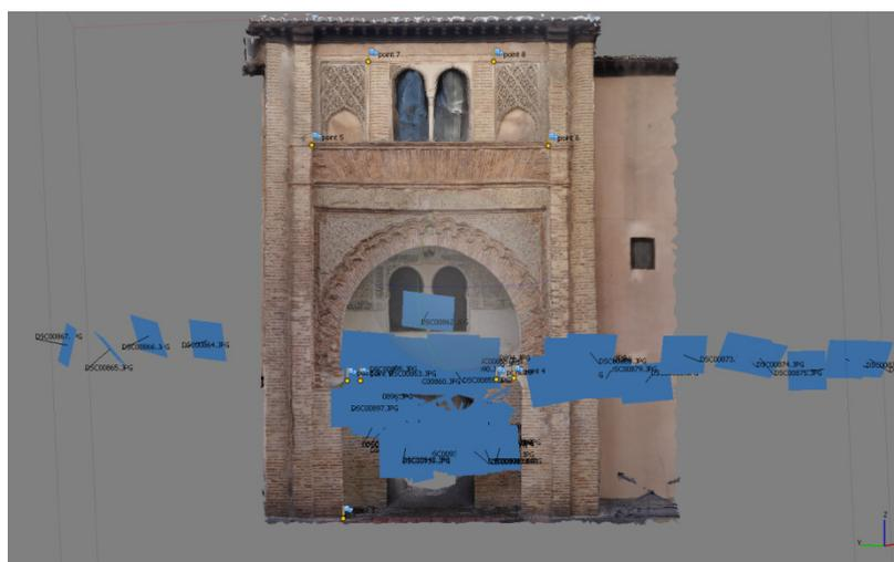
**Figure 10.** Photogrammetry: structure from motion computed for the Corral del Carbón entrance (every photograph used in the entrance survey is represented by a blue rectangle placed in its 3D position).
