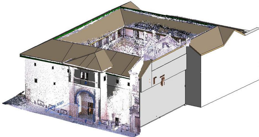
**Figure 12.** Corral del Carbón Heritage Building Information Modeling (HBIM) overlapping the scanned point cloud.
