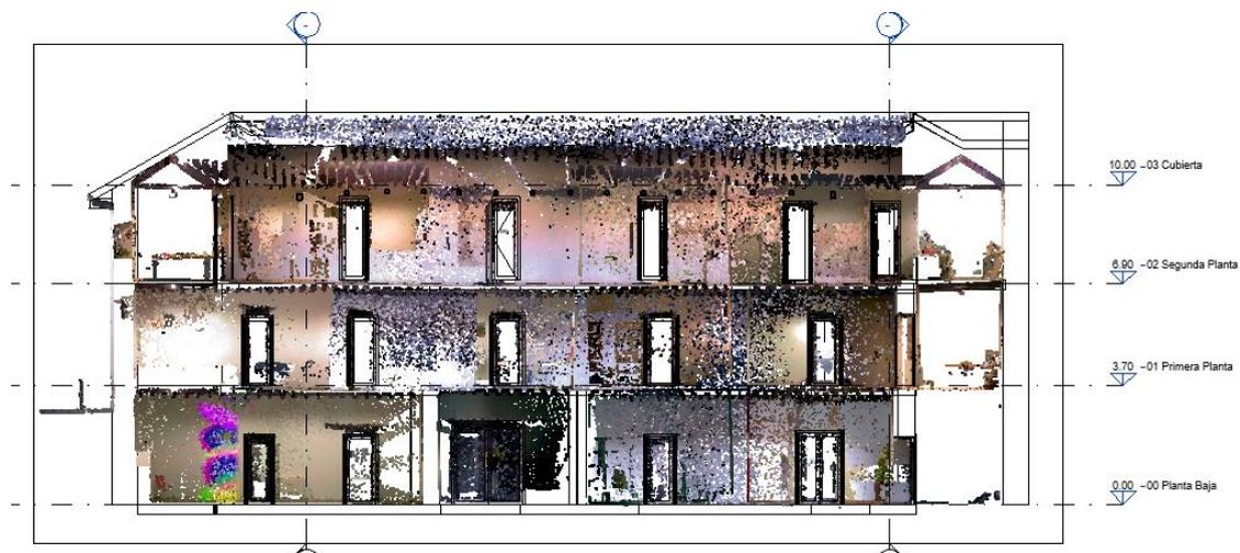
**Figure 17.** Elevation derived from the point cloud.
