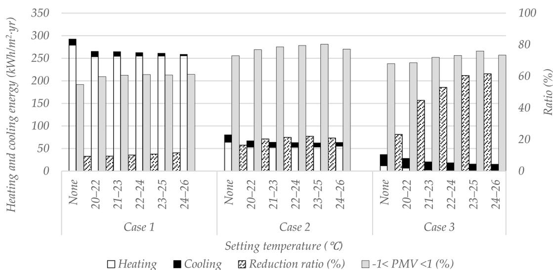
Figure 7. Annual heating and cooling load by the PCMs; 2nd simulation.
