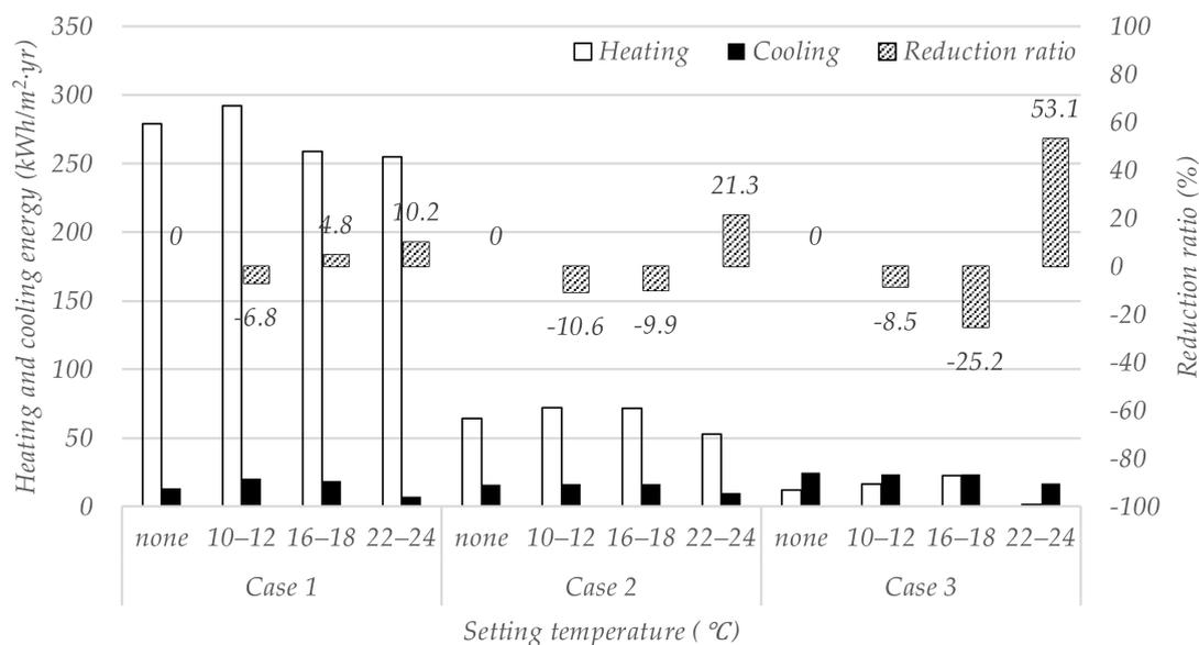
Figure 6. Annual heating and cooling load by the PCMs; 1st simulation.
