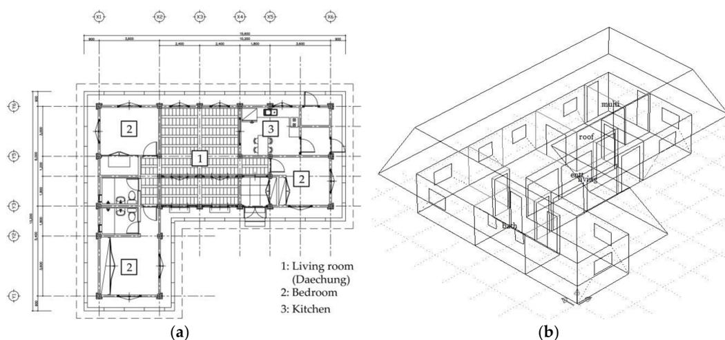
**Figure 3.** Drawing of the proposed *Hanok* (a) Floor Plan [41]; (b) 3-d perspective view of the energy simulation modeling.
