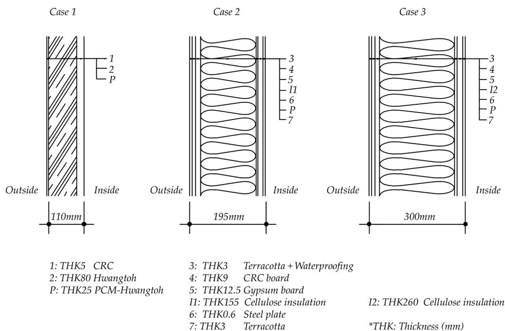
**Figure 4.** Section drawing detail of PCM-*Hwangtoh* composites installation.
