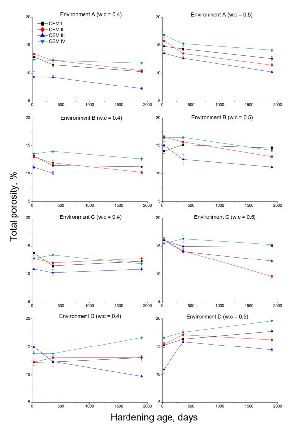
Figure 1. Results of total porosity for the studied mortars.
