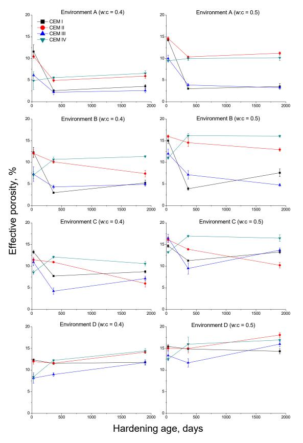
Figure 8. Effective porosity results for the studied mortars.
