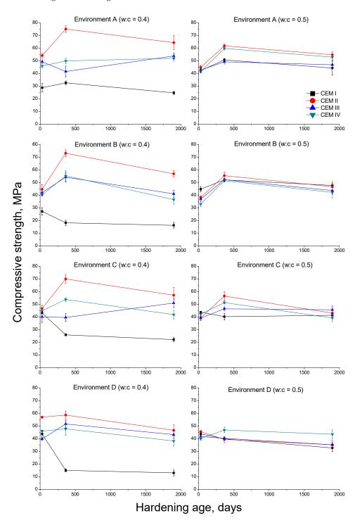
Figure 10. Results of compressive strength for the studied mortars.
