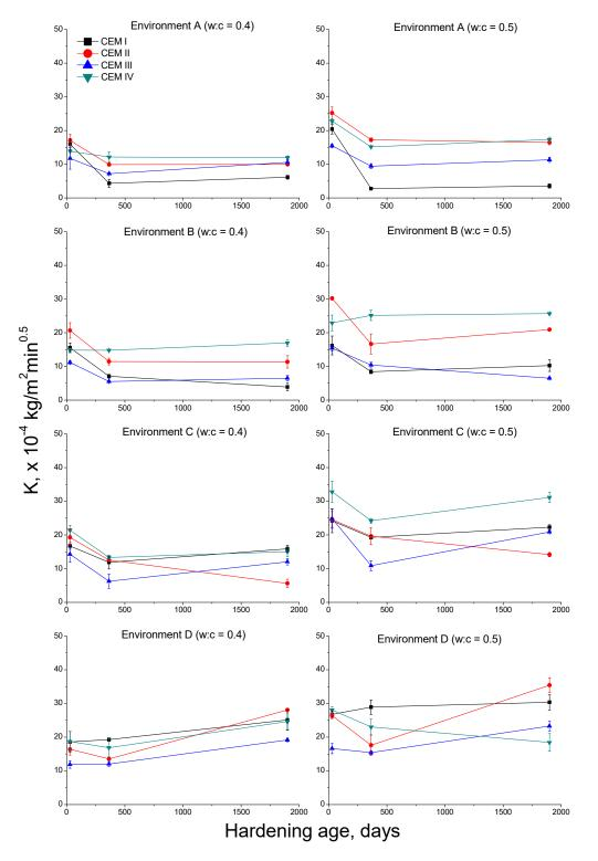
Figure 7. Results of capillary suction coefficient (K) for the studied mortars.
