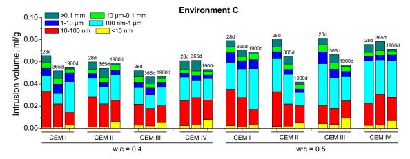
Figure 4. Pore size distributions obtained for environment C.
