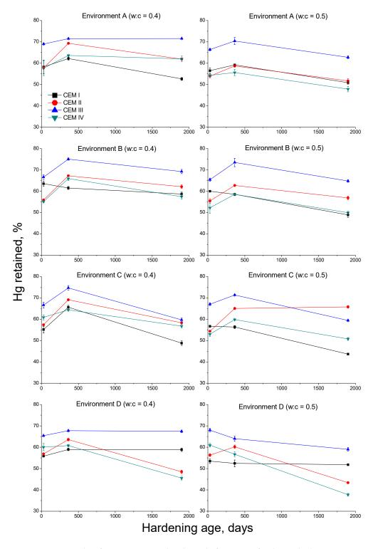
Figure 6. Results of mercury retained at the end of MIP tests for the studied mortars.
