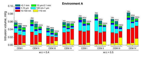
Figure 2. Pore size distributions obtained for environment A.
