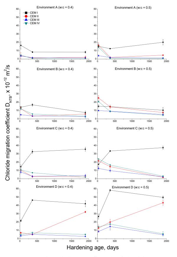
Figure 9. Non-steady-state chloride migration coefficient evolution for the studied mortars.
