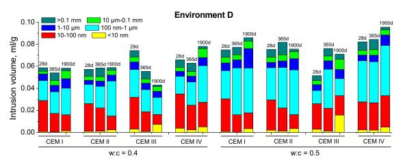
Figure 5. Pore size distributions obtained for environment D.
