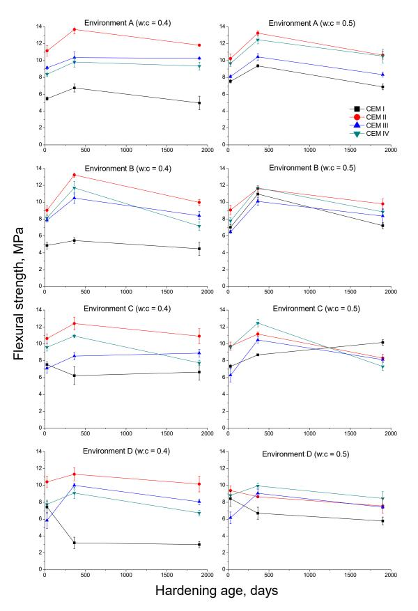
Figure 11. Results of flexural strength for the studied mortars.
