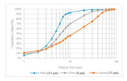
Figure 1. Limestone powder particle size distribution by mass.
