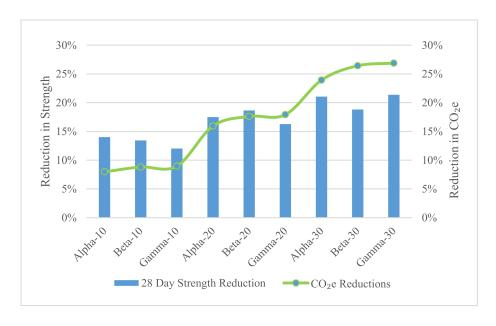
Figure 13. % CO<sub>2</sub>e Reductions Compared to % Strength Reduction.
