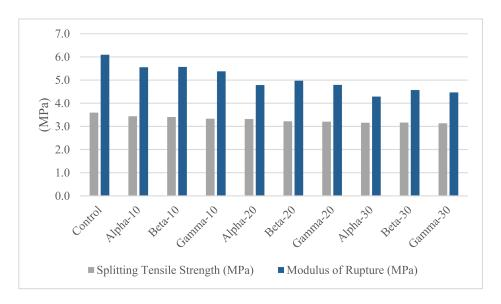
Figure 3. Twenty-eight day splitting tensile strength and flexural strength.
