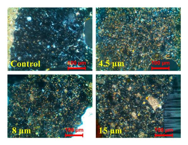
Figure 7. Images of control and concrete with limestone powder.
