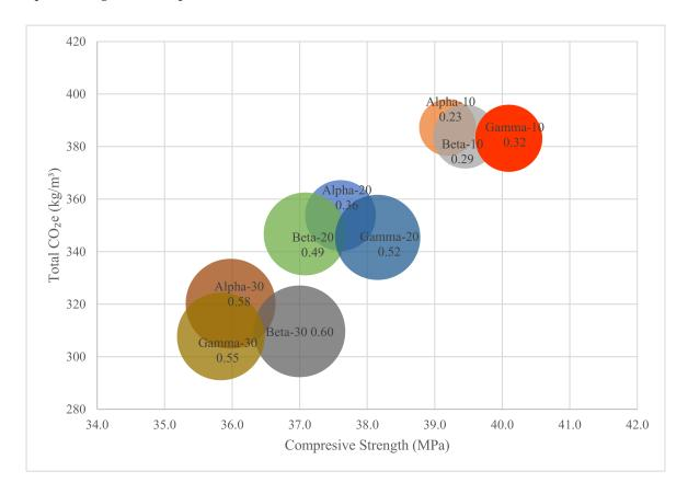
Figure 14. Optimizing the limestone powder in concrete at 28 Days.
