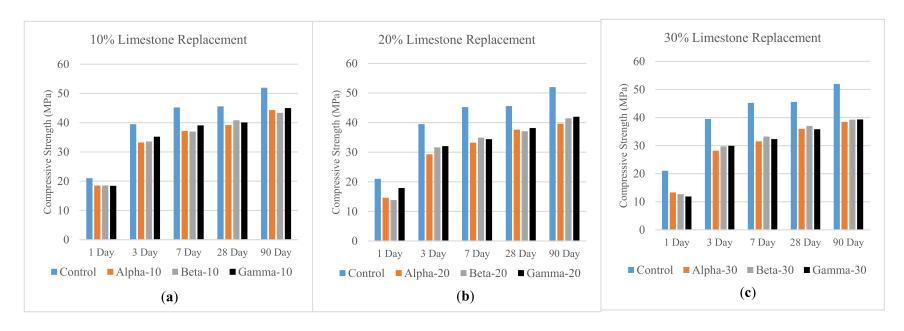
**Figure 2.** Effects of limestone powder on compressive strength.
