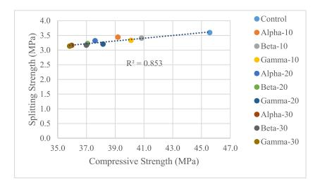
Figure 4. Correlation of splitting tensile strength and compressive strength.
