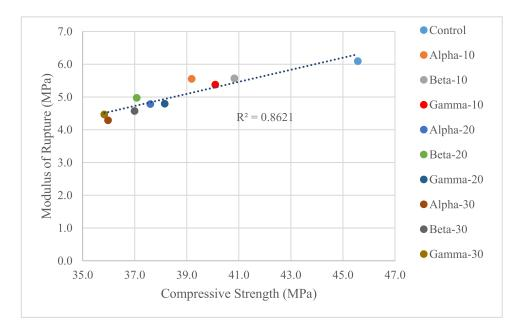
Figure 5. Correlation of modulus of rupture and compressive strength.
