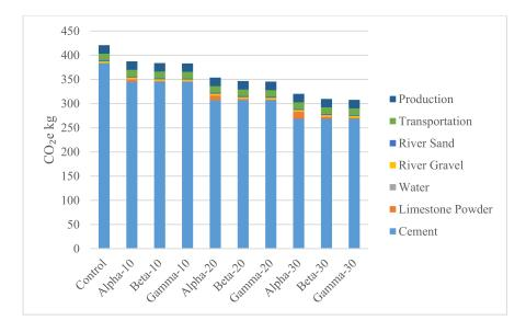
Figure 12. CO<sub>2</sub>e Emission per m<sup>3</sup> of concrete.
