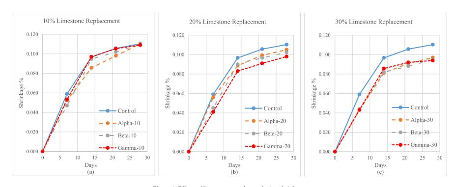
Figure 6. Effects of limestone powder on drying shrinkage.
