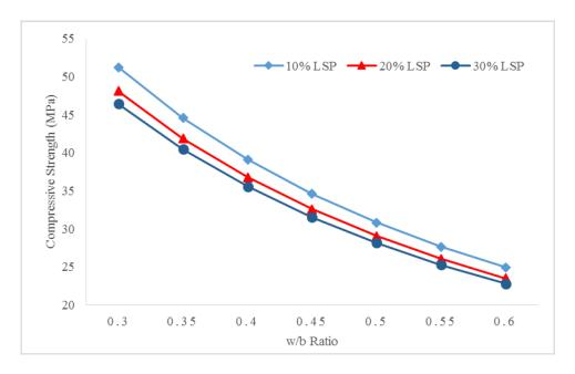
Figure 11. Limestone powder prediction model with different w/b ratios.
