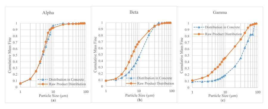
Figure 9. Limestone powder particle distribution in concrete.
