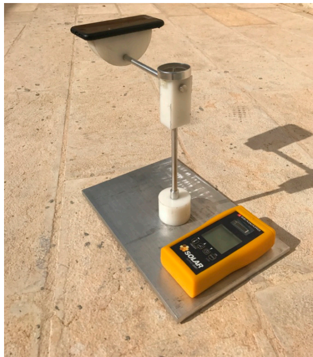
Figure 3. Setup orientation, smartphone pointing north and rotating toward south.
