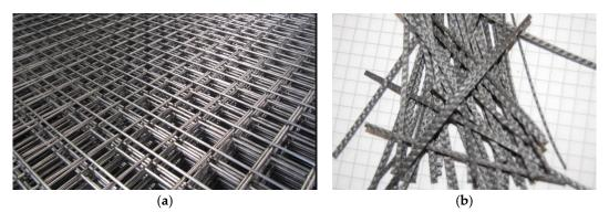
Figure 1. Visual aspect of the two different reinforcements: (a) steel mesh; (b) polyolefin fibres.
