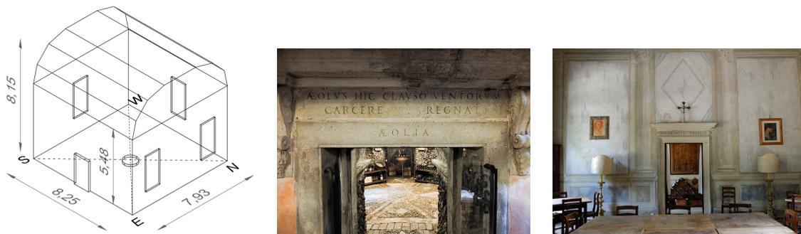
**Figure 10.** 3D geometry of Apollinea hall (left). The letters indicate the cardinal points. The room has four windows, the access door on the south-east wall, and a marble vent on the floor [50]. The inscription over the access door to the Carcere dei Venti (Aeolus hic clauso ventorum carcere regnat, Eolia) (center). The interior of Apollinea hall (right).
