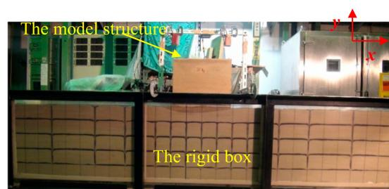
Figure 1. Shaking table with experimental set up.
