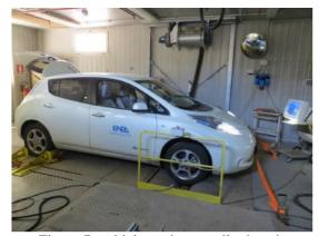
Figure 7: vehicle testing at roller bench
