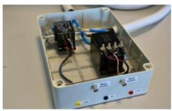
Figure 6: LEM DC output sensors
