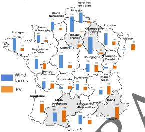
Figure 1: installed wind and PV power capacities by area in France (MW). Extracted from [17]
