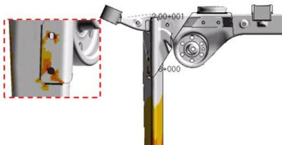
Figure 12: Analysis results for torsion beam axle
