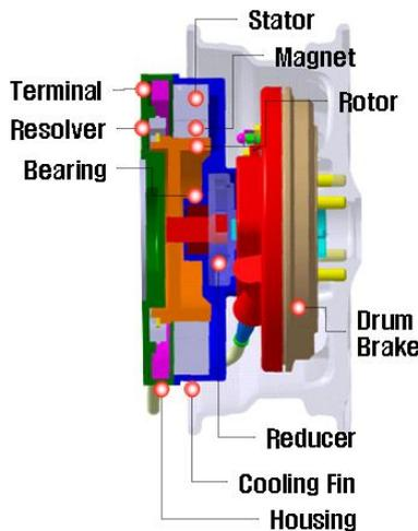
Figure 3: Cross section of In-Wheel motor
