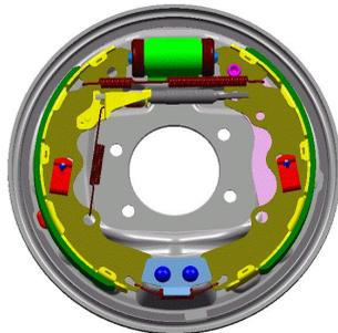
Figure 8: Schematic diagram of drum brake
