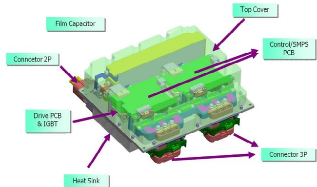
Figure 6: Composition of integrated inverter
