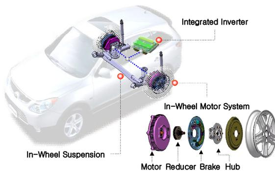
Figure 1: Configuration of In-Wheel system
