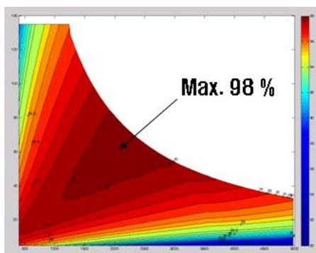
Figure 5: Efficiency map of In-Wheel motor
