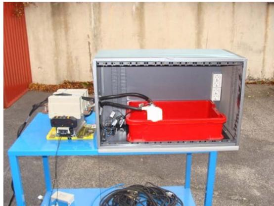
Figure 2. The test setup for short circuit test.
