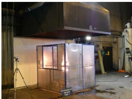
Figure 7. The test set-up during a fire test. The test set-up was enclosed with a safety net cage and the HRR, i.e. the power in kW from the fire, was measured using a 2 MW furniture calorimeter.
