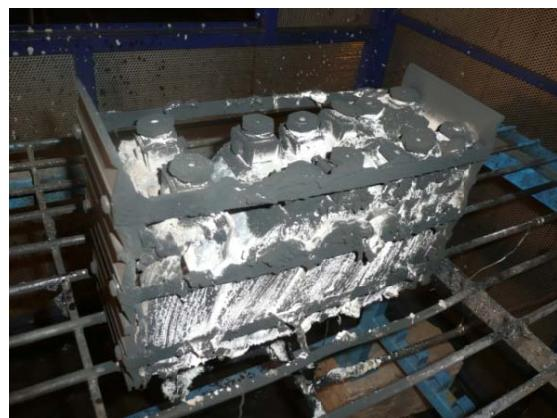
Figure 9. The same battery as in Figure 8, after performed fire test.
