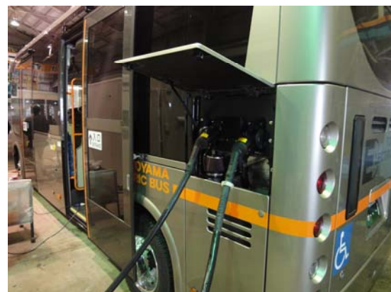
Figure 5 : Connector used for charging the bus.
