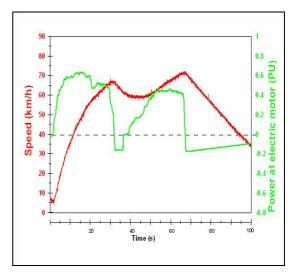
Figure 3: Normalized power at the electric motor, as well as the speed profile of the bus. It can clearly be seen that with increasing speed, the motor is delivering power to the wheels (positive). While slowing down, the motor delivers power back to the propulsion system (negative).
