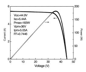
Figure 5: I-V characteristics curves of PV module
