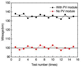
Figure 6: comparison of the driving range for SEV with and no PV module
