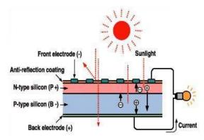
Figure 1: typical schematic diagram of the solar cell
