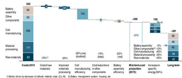
Figure 6: Cost reduction levers in the battery value chain [USD/kWh] and necessary increase of specific energy
