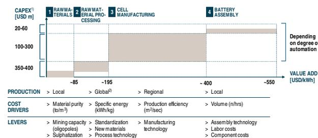
Fig. 5: Value chain EV battery (high – "Ternary mix" LiNi<sub>x</sub>Co<sub>x</sub>Mn<sub>x</sub>O<sub>2</sub>, 2010)
