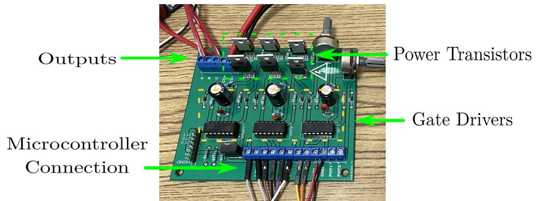
**Figure 11.** Experimental 6-pulse electronic speed controller for brushless DC motor evaluation.
