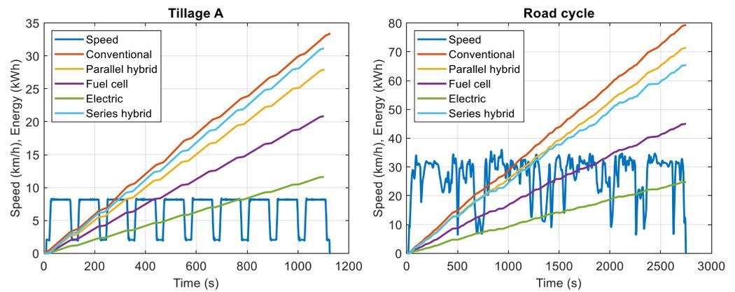
**Figure 8.** Cumulative energy consumption in the Tillage A and Road cycles for the medium-sized tractor models.
