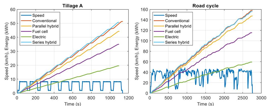
**Figure 7.** Cumulative energy consumption in the Tillage A and Road cycles for the large-sized tractor models.
