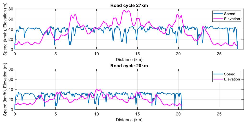
**Figure 5.** Measured and generated road cycles for tractor-trailer simulations.
