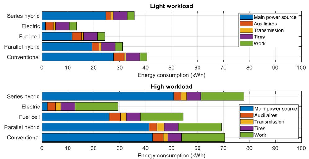
**Figure 13.** Distribution of energy losses for the different large tractor models in the Tillage A cycle with two workloads.
