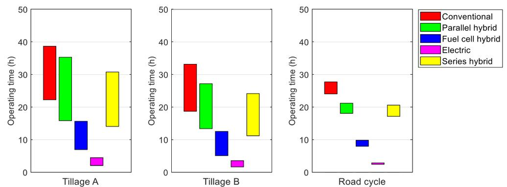
**Figure 15.** Calculated variations in operating times for different cycles for the large-sized tractor.
