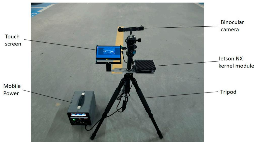
Figure 8. System hardware design.
