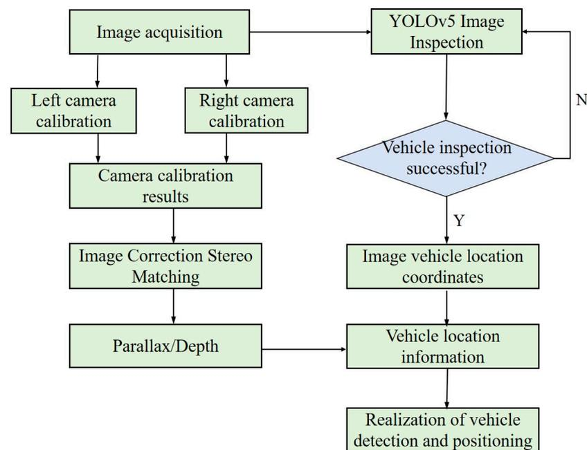
**Figure 9.** System software design flowchart.
