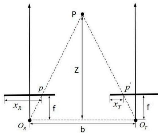
**Figure 5.** Schematic diagram of binocular positioning.
