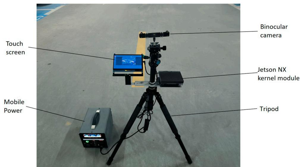
Figure 8. System hardware design.
