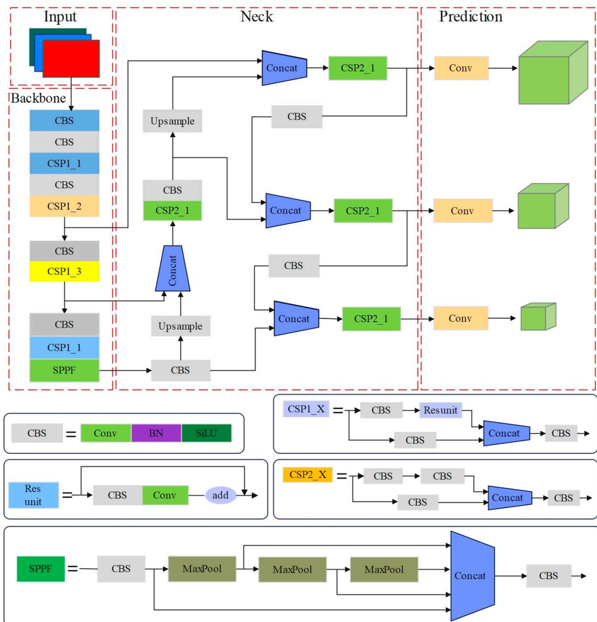
Figure 1. YOLOv5 network structure diagram.
