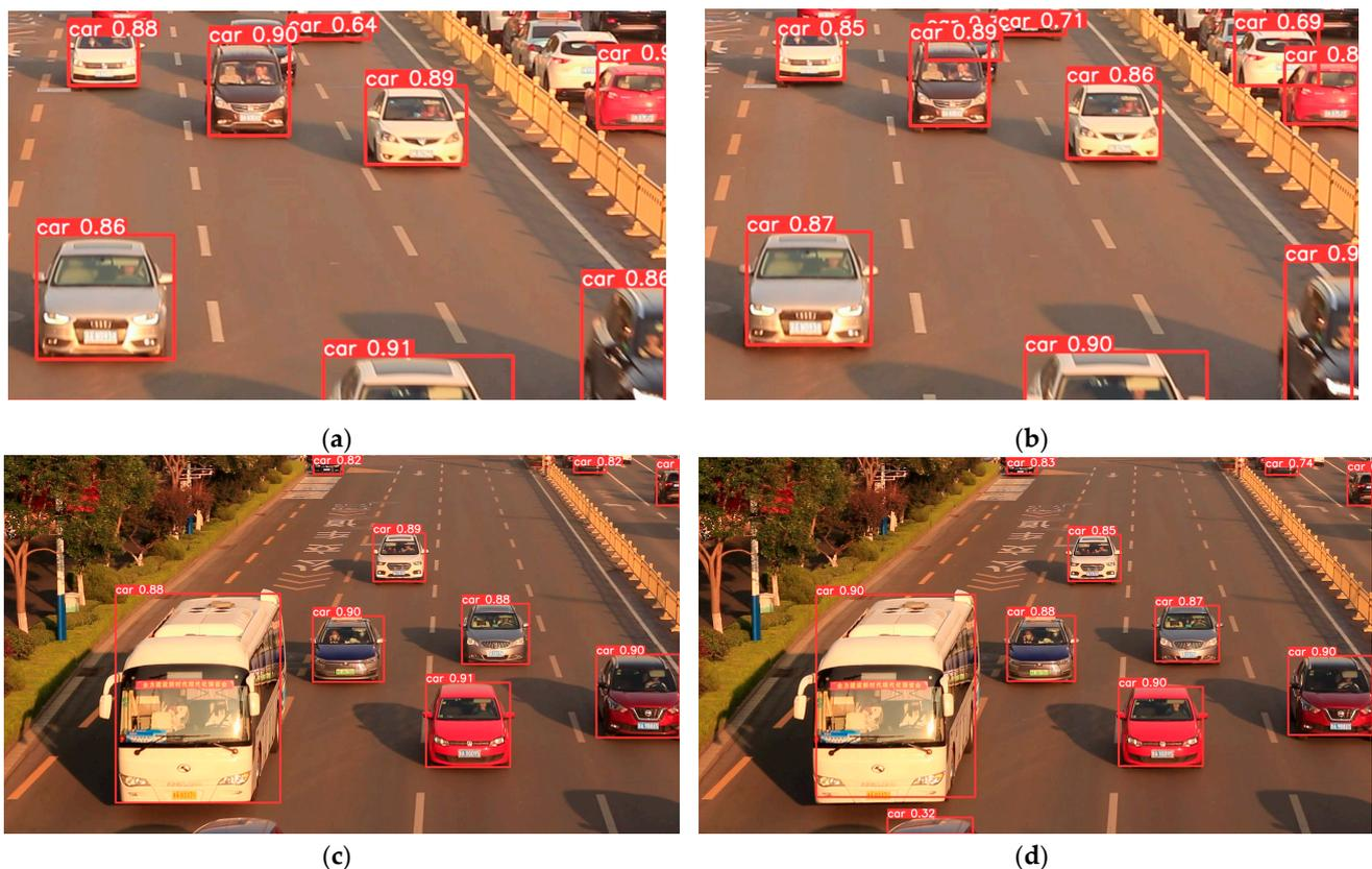
**Figure 11.** Vehicle detection and localization effect diagram. (a,c) The effect of unimproved detection; (b,d) the effect of improved detection.
