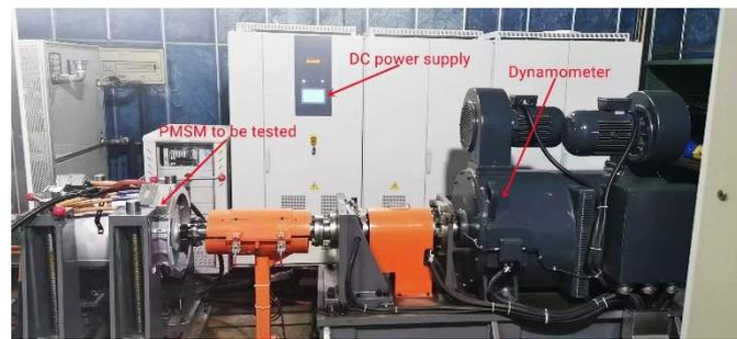
**Figure 6.** Physical picture of test bench.
