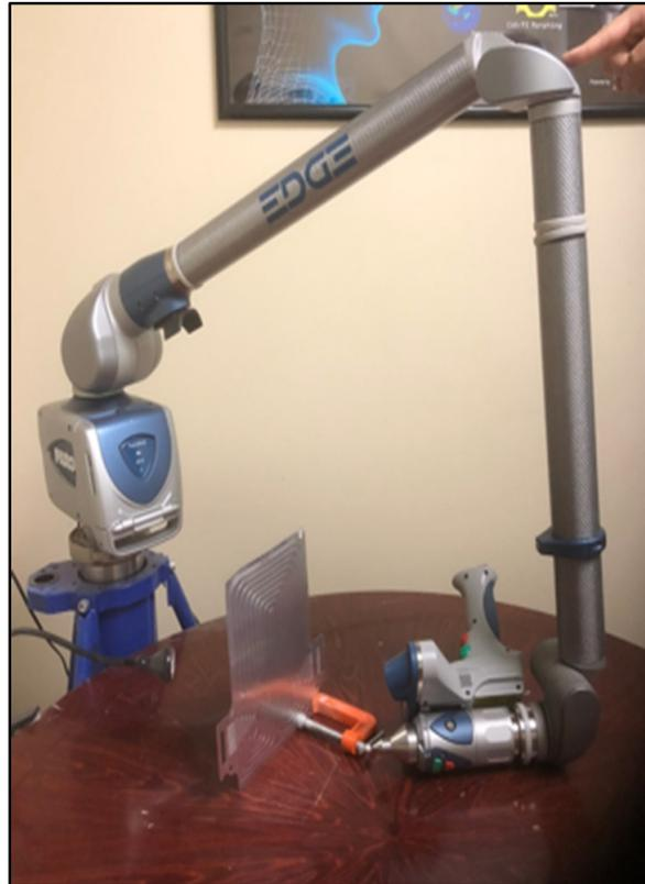
**Figure 1.** 3D Laser scanning of microchannel cold plate used for cooling the lithium-ion battery.
