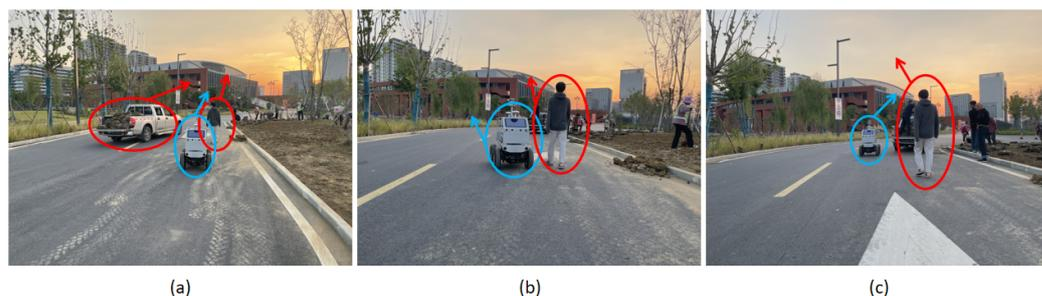
**Figure 22.** Dynamic obstacle avoidance in the park scene: (a) when the robot is far away from pedestrians; (b) the robot avoids pedestrians; (c) the robot continues to perform navigation tasks.
