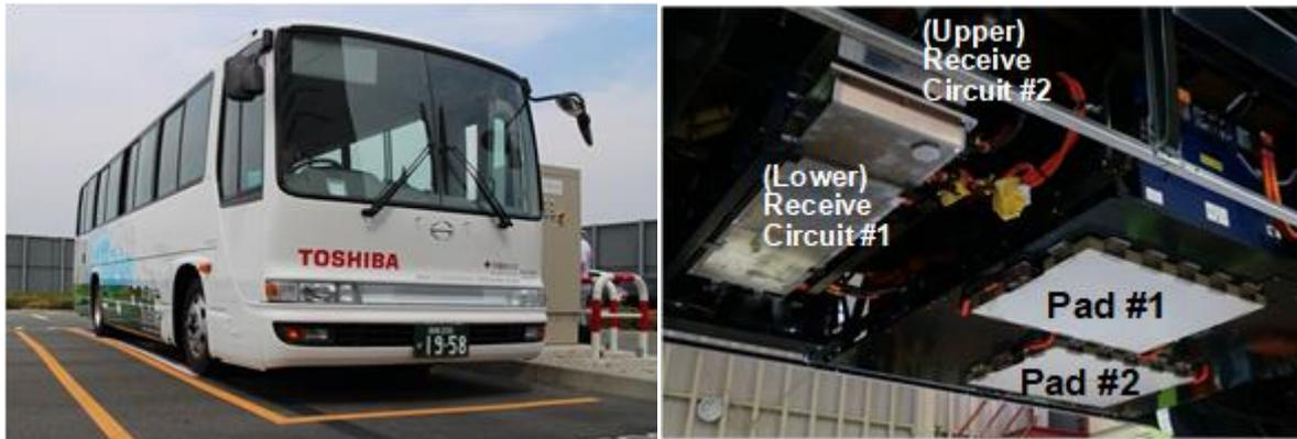
Figure 7. The medium-size bus and the receiving equipment installed on the bus.
