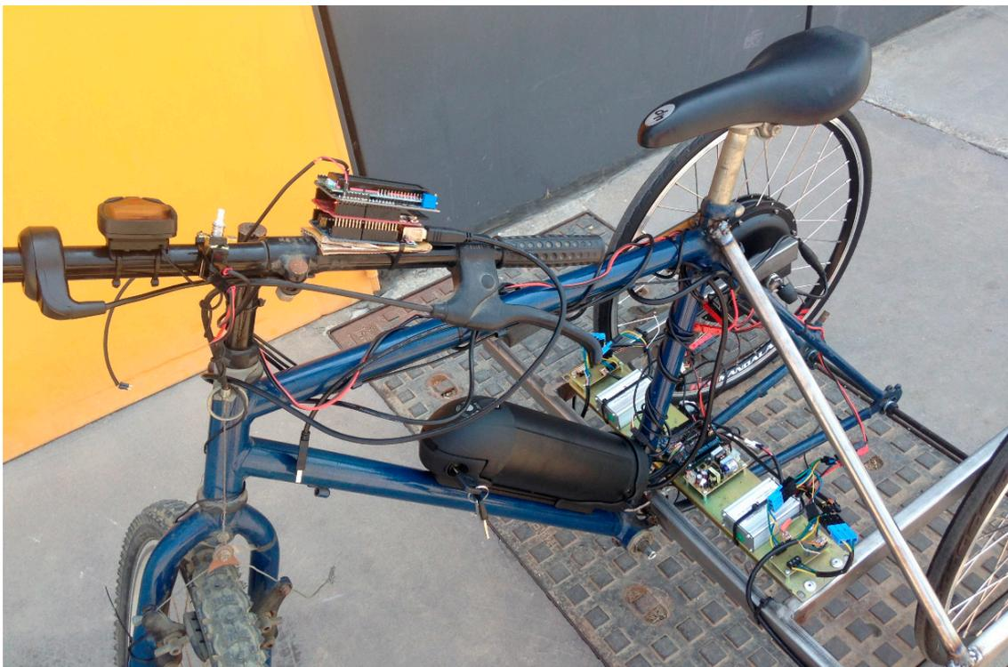
**Figure 2.** Three-wheel light electric vehicle (LEV) system generated reconditioning a common bicycle. Modifications: Two driving rear wheels with motors integrated; ED and power controllers placed in an added back platform and a battery pack placed in the original frame behind the driver.
