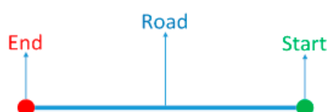
Figure 4. A road (edge) feature only has one start point and one end point, but no break point.
