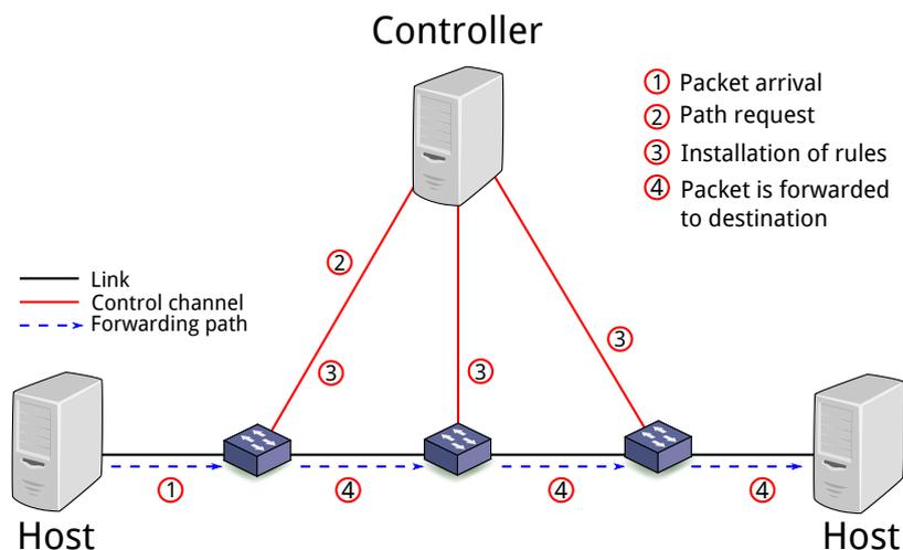
The mechanisms to enable reactive flow management in OpenFlow are based on timeouts. The controller sets an expiry timer that defaults to one second. The switch tracks the duration to the last match for all entries. Unused entries are removed from the switch. When more packets of an expired flow arrive, the controller must be queried for path installation again.
