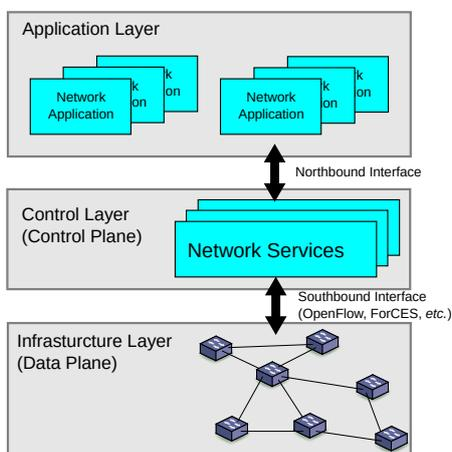
Figure 1 illustrates the SDN framework, which consists of three layers. The lowest layer is the infrastructure layer, also called the data plane. It comprises the forwarding network elements. The responsibilities of the forwarding plane are mainly data forwarding, as well as monitoring local information and gathering statistics.
