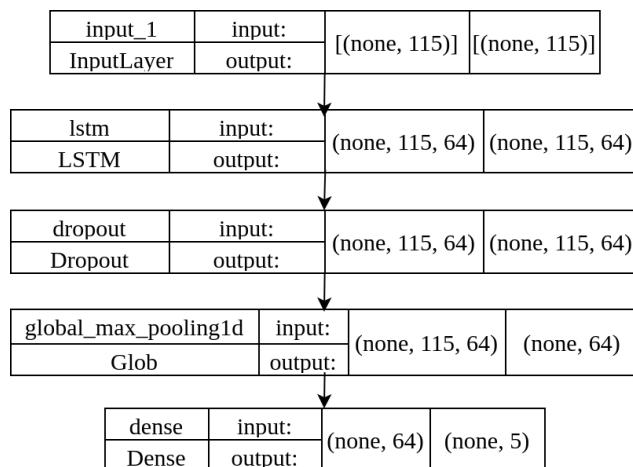
**Figure 5.** LSTM model architecture.
