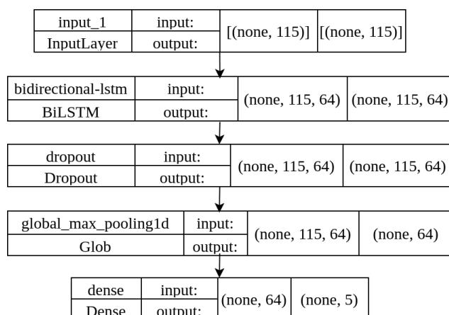
**Figure 6.** BiLSTM model architecture.
