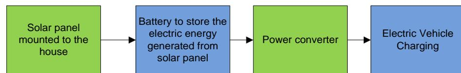
**Figure 7.** Solar panel and charging system for household purposes.
