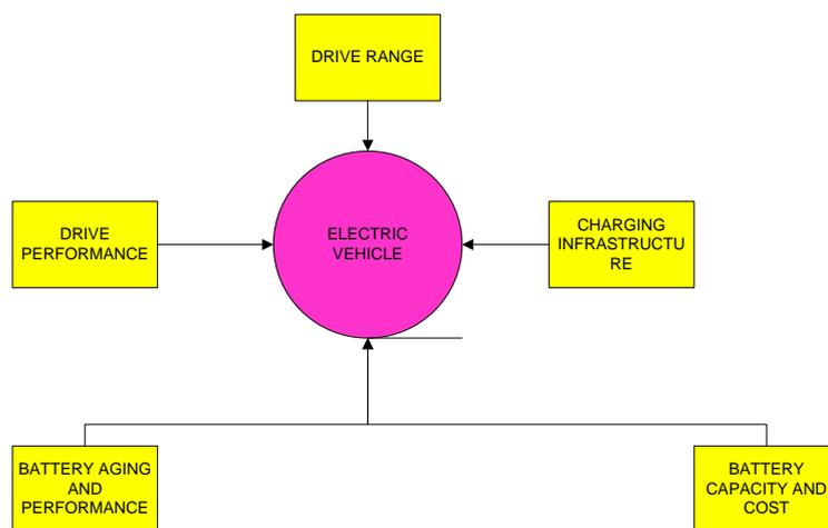
**Figure 3.** Parameters affecting EV overall performance.
