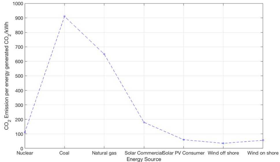
**Figure 4.** CO<sub>2</sub>/kWh generated from different energy sources.
