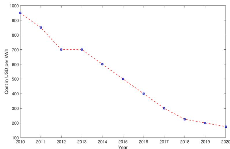
**Figure 12.** Li-Ion battery cost per kWh over years from 2010.
