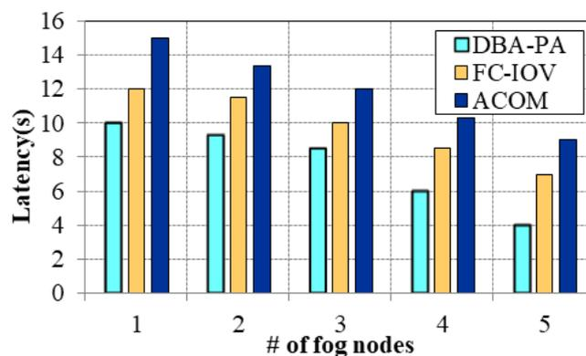
Figure 12. Number of Fog Nodes vs. Latency.
