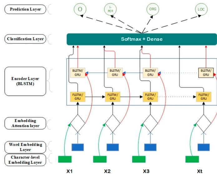
**Figure 1.** Main architecture of the network. Word embedding is provided to a Bi-LSTM/GRU. The forward unit represents the word  $X_t$  and its left context, whereas the backward unit represents the word  $X_t$  and its right context. Concatenating the two vectors yields a representation of the word  $X_t$  and its context, and this embedded representation is fed to the classification layer.
