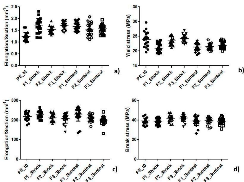
**Figure 2.** Trend of (a) yield strain; (b) yield stress; (c) break strain; and (d) break stress values obtained from all samples.
