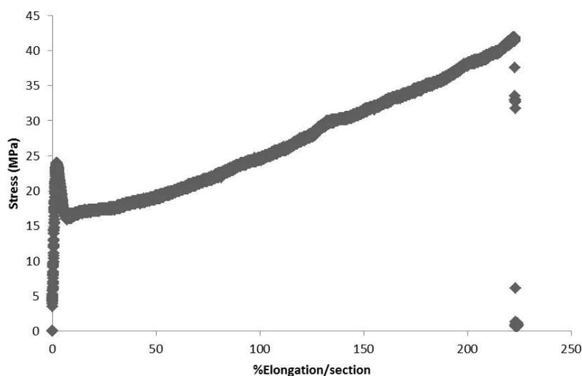
**Figure 1.** Example of a diagram obtained from the tensile test of the packaging.
