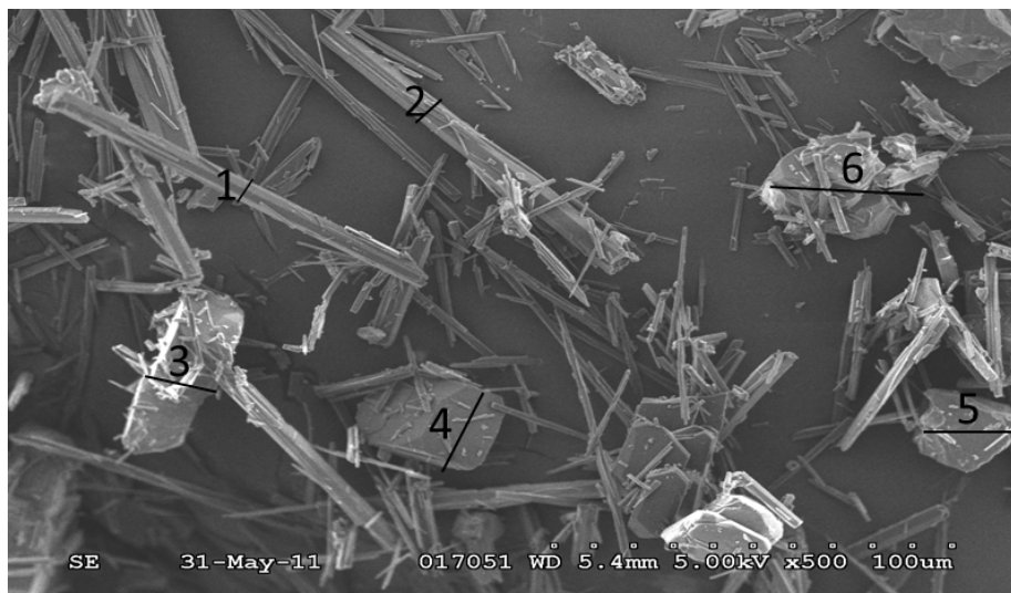
Figure 9. SEM picture of the sample taken at 20 min in Run 2. Crystals 1 and 2 are considered to be Form II and 3-6 as Form III.
