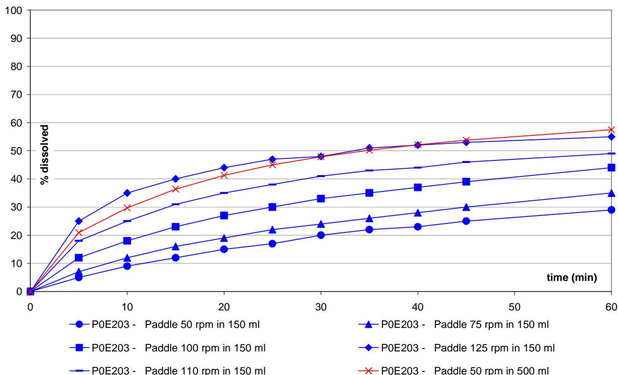
For salicylic acid non-disintegrating tablets (Figure 3), a small vessel/paddle at 150 rpm results in a similar profile to the USP paddle 100 rpm method (sf = 1.5).
