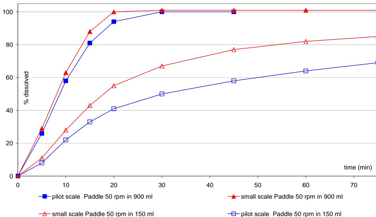
**Figure 8.** IR(2) tablets: comparison after storage using small vessel accessories.
