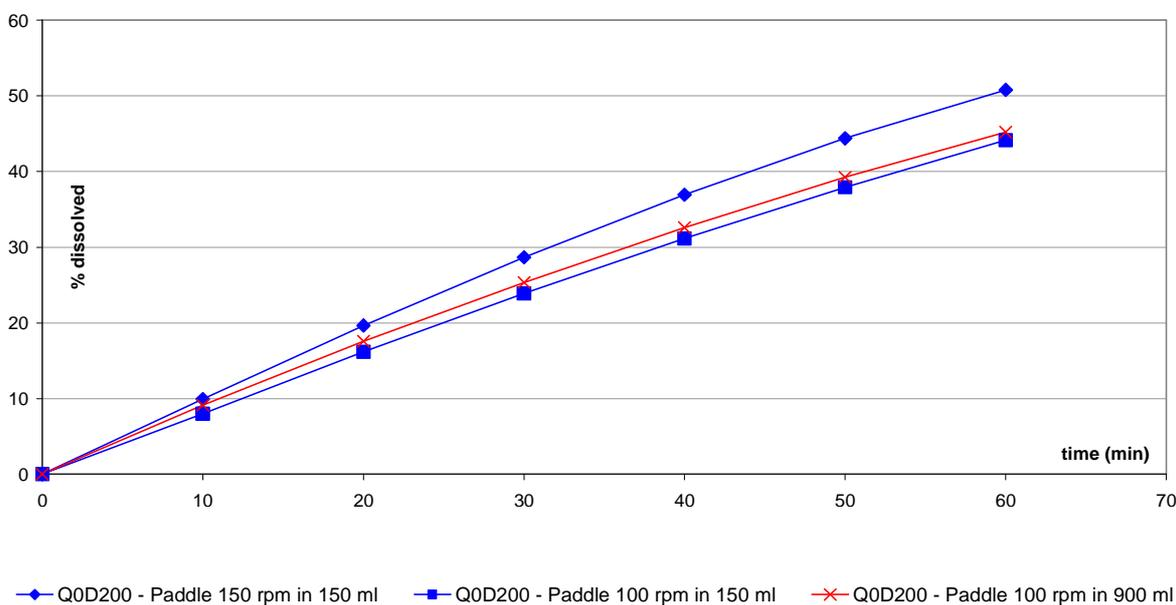
For the extended release tablets ER4H and ER8H (Figure 4), the impact of the small vessel/paddle setup is less pronounced. By varying the rotation speed from 50 to 100 rpm, similar profiles can be observed and the ratios remain very close.
