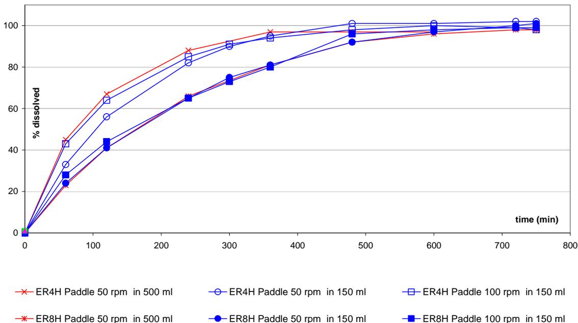
For the IR(1) tablets (Figure 5), both motion speeds of 100 rpm and 125 rpm when using the small vessel/paddle resulted in a similar profile to the one liter method with paddle at 50 rpm ( $sf = 2.5$ ).
