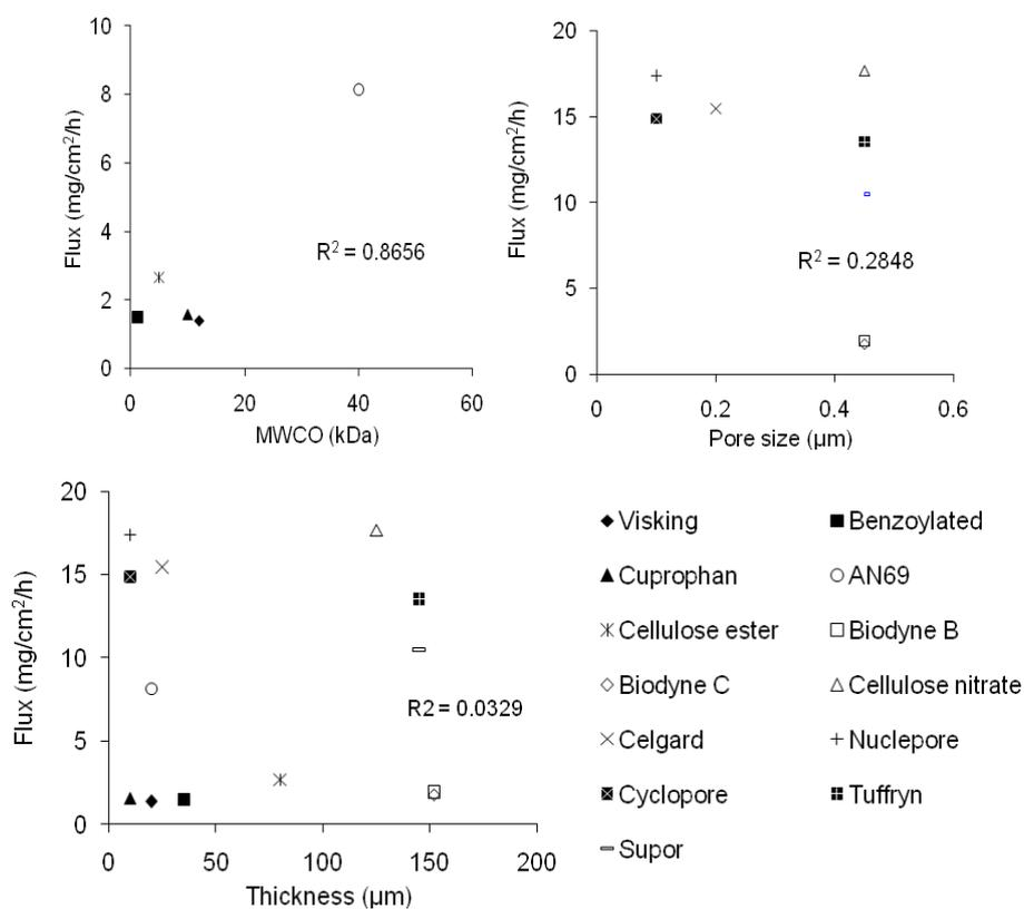
Pore sizes were correlated within high-flux membranes and MWCO were investigated within low-flux membranes using correlation regression analysis. The cumulative ibuprofen drug diffusion *versus* time plot through membranes of different pore sizes and surface groups are showed in Figure 3 (a) and (b), respectively. There was no statistical significance between ibuprofen fluxes over six hours when using membranes of different pore sizes or surface groups.
