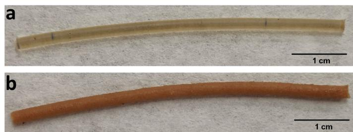
**Figure 2.** Digital pictures of (a) extruded HPMCAS-HG filament, (b) extruded drug-loaded PVA filament.
