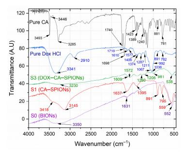
Figure 6. FTIR spectra of BIONs, CA-SPIONs, DOX-CA-SPIONs, magnetite, and citric acid.
