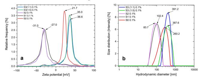
**Figure 1.** (a) Zeta potential and (b) size distribution of particle agglomerates for neutral pH (6.5) at concentrations of 0.1% w/v. S0: bare iron oxide nanoparticles; S1: CA-modified iron oxide nanoparticles (IONPs); S2: CA-modified and electrohydraulic discharge-processed IONPs; S3: CA-modified and DOX-loaded IONPs.
