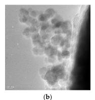
**Figure 4.** TEM images of CA-modified iron oxide nanoparticles at different magnifications (scalebars are 50 nm (**a**) and 10 nm (**b**)).
