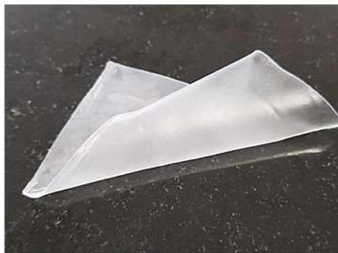
**Figure 2.** A thick film was rolled up to assess its flexibility.
