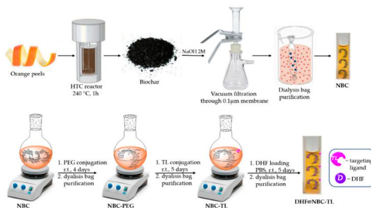
**Figure 2.** Schematic representation of methodology employed for the preparation of NBC-based DDS.
