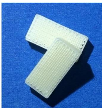
**Figure 2.** Picture of printed objects (3 × 15 × 7.5 mm) using in-house-produced filaments based on EC and HPMC for the evaluation of uniformity of mass according to Ph.Eur. 2.9.5.
