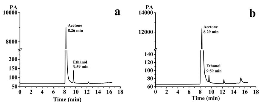
**Figure 7.** (a) Gas chromatograms of ethanol standard solution; (b) The gas phase of the 100 mg/mL acetone solution of HK–PLX (1:4) SD.
