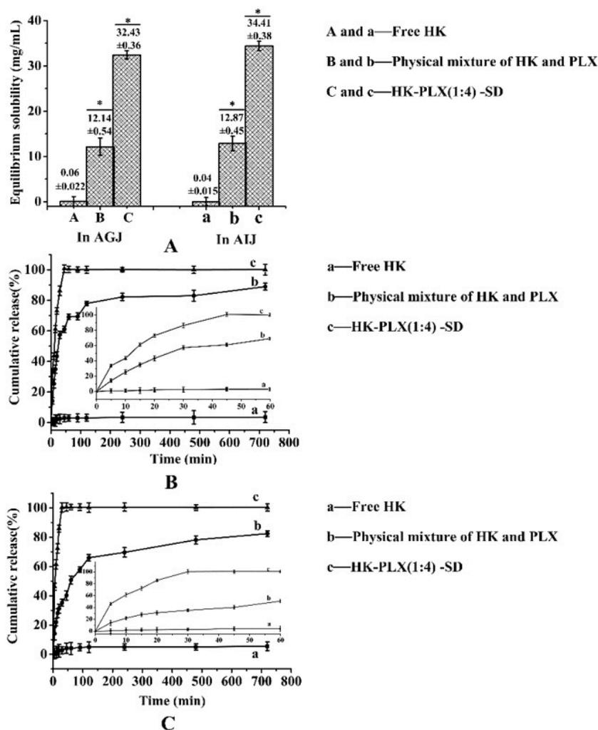
**Figure 8.** Equilibrium solubility (\*  $p < 0.05$ ) (A) and the release profiles in artificial gastric juice (B) and artificial intestinal juice (C) for free HK, the physical mixture, and the HK-PLX (1:4) SD.
