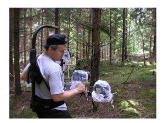
Figure 2. The five-camera rig in the field with rain covers, carried with EasyRig 2.5.
