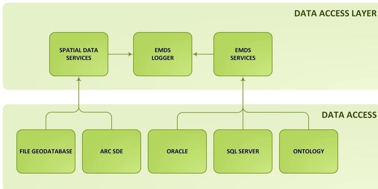
**Figure 3.** Data Services Tier. Data storage functionality is hidden behind services and objects that are accessed by the Business Logic Tier (Figure 4).
