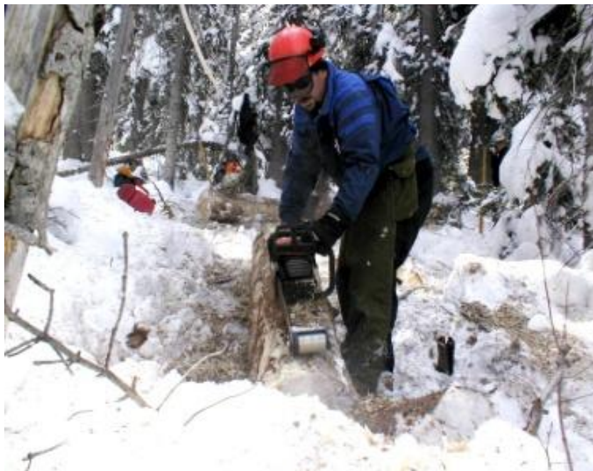
Figure 6. Log Wizard™ [211] used to peel bark from spruce beetle infested Engelmann spruce (Photo: A. Steven Munson).
