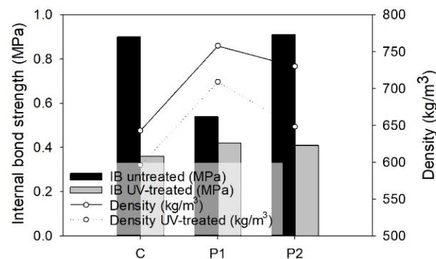
**Figure 10.** Internal bond strength and density results, obtained from the internal bond strength test, for each of the UV-treated samples and untreated samples of the control PB and PB-bbwas.
