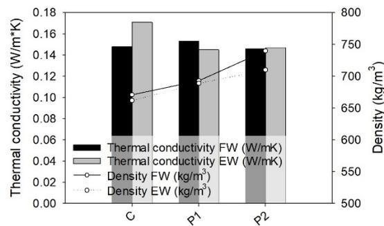
**Figure 12.** Thermal conductivity and density, obtained from the thermal conductivity test, for each of the flatwise and edgewise positions of the control PB and PB-bbw as.
