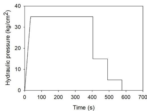
**Figure 1.** Hot three-stage pressing cycle for control PB samples.
