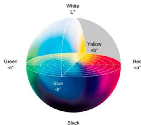
**Figure 3.** Model for objective color measurement of the International Commission on Illumination (CIELAB). Its color coordinates,  $L^*a^*b^*$ , describe lightness: brightness ( $L^*$ ) and black ( $L^*-$ ), and the colors: red ( $a^*$ ), green ( $a^*-$ ), yellow ( $b^*$ ), and blue ( $b^*-$ ) [22].
