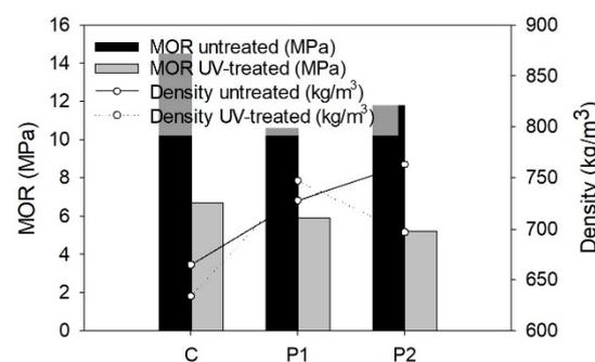
**Figure 7.** MOR and density results, obtained from the bending test, for each of the UV-treated samples and the untreated samples of the control PB and the PB-bbw as.
