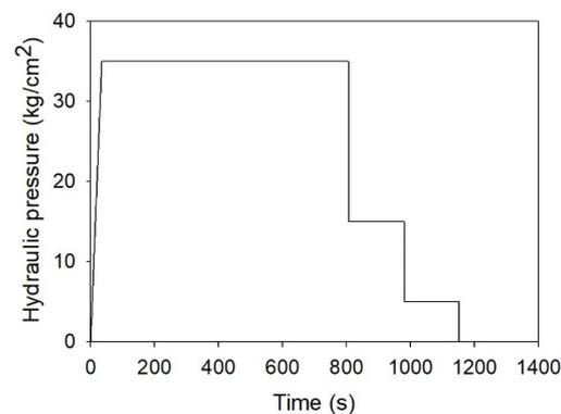
**Figure 2.** Hot three-stage pressing cycle for samples based on bio wood adhesives.
