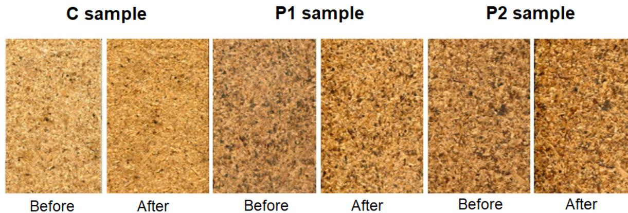
**Figure 4.** Results of C, P1, and P2 samples before and after exposure to an accelerated UV aging.
