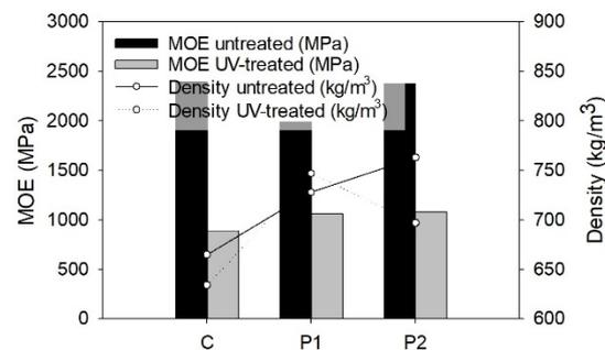
**Figure 6.** MOE and density results, obtained from the bending test, for each of the UV-treated samples and the untreated samples of the control PB and the PB-bbw as.
