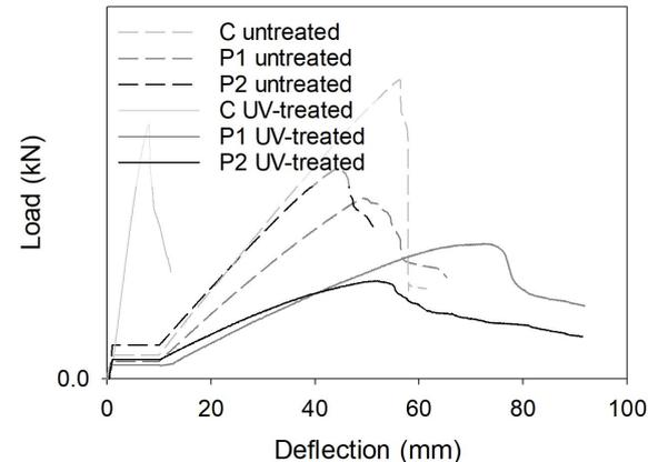
**Figure 8.** Load deflection curves, obtained from the bending test, for each of the UV-treated samples and the untreated samples of the control PB and the PB-bbwa.
