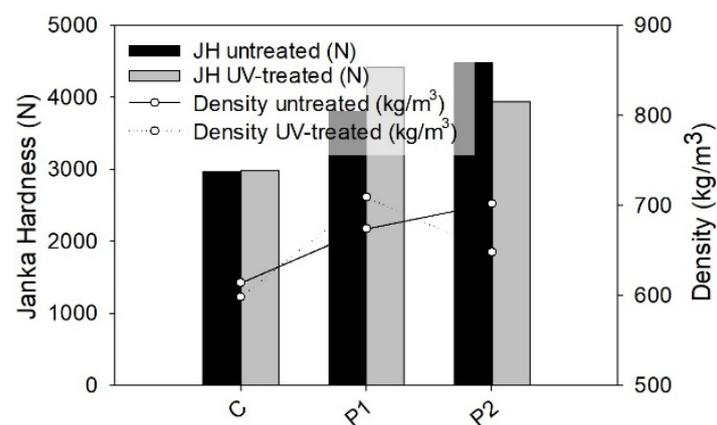
**Figure 11.** Hardness and density, obtained from the Janka hardness test, for each of the UV-treated samples and the untreated samples of the control PB and PB-bbwas.
