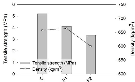
**Figure 9.** Tensile strength and density results, obtained from the tensile strength test, of each control PB and PB-bbwa sample.
