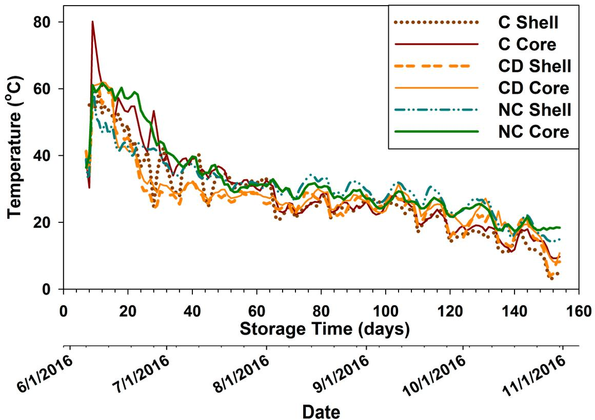
**Figure 3.** Daily mean temperature in the core (about  $\frac{1}{2}$  depth) and shell (<45-cm depth) of C, NC, and CD piles of willow and poplar wood chips (NC—no cover on pile; C—covered pile; CD—covered pile with dome ventilation).
