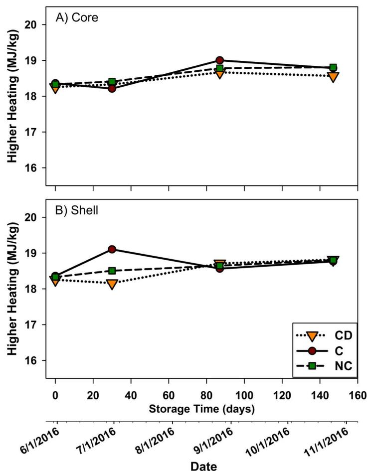
**Figure 5.** Variation of the higher heating value of willow and poplar wood chips stored for five months in piles with three different treatments (NC—no cover on pile; C—covered pile; CD—covered pile with dome ventilation); (A) samples from the core; (B) samples from the shell.
