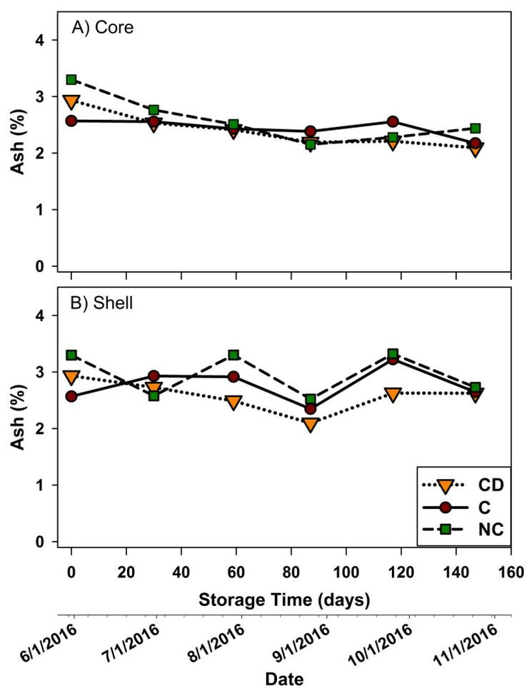
**Figure 7.** Variation of the ash content of willow and poplar wood chips stored for five months in piles with three different treatments (NC—no cover on pile; C—covered pile; CD—covered pile with dome ventilation); (A) samples from the core; (B) samples from the shell.
