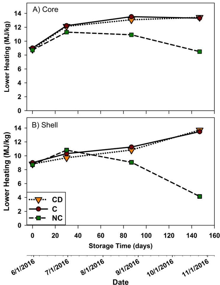
**Figure 6.** Variation of the lower heating value of willow and poplar wood chips stored for five months in piles with three different treatments (NC—no cover on pile; C—covered pile; CD—covered pile with dome ventilation); (A) samples from the core; (B) samples from the shell.
