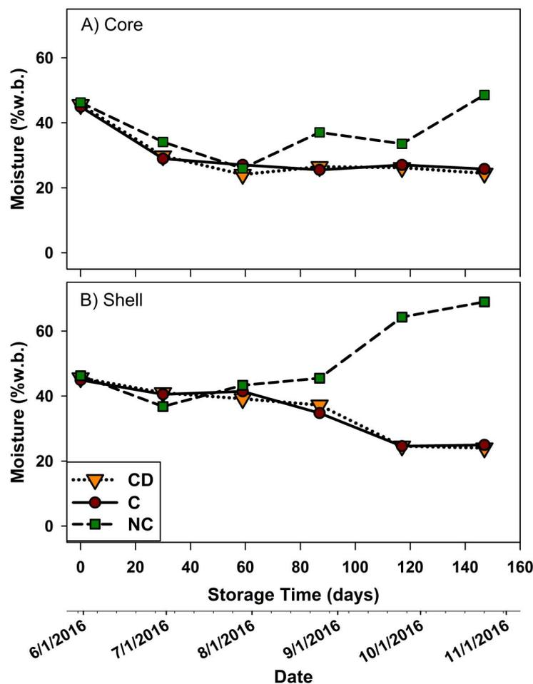
**Figure 4.** Variation of the moisture content of willow and poplar wood chips stored for five months in piles with three different treatments (NC—no cover on pile; C—covered pile; CD—covered pile with dome ventilation); (A) samples from the core; (B) samples from the shell.
