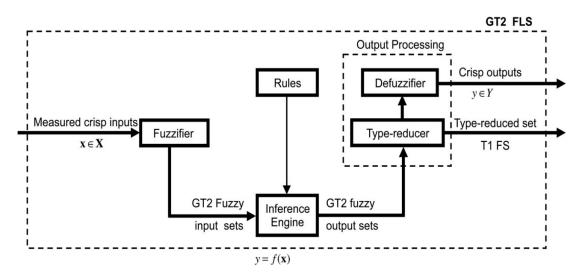
Figure 1. Structure of a GT2 FLS, with permission from [9].
