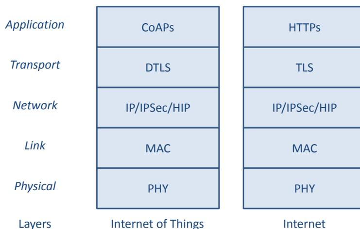
It is important to observe that the IoT protocol suite depicted in Figure 2 represents just the possible choices to enforce data protection (at different layers) by a smart object, rather than the actual set of security mechanisms effectively implemented and simultaneously used at different layers. At the opposite, in order to minimize the used resources, particular attention has to be devoted to avoid the repetition of the same functionalities at different layers, if not strictly required.
