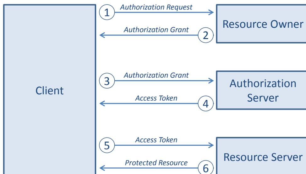
The OAuth authorization framework (currently in version 2.0 [77]) enables a third-party application to obtain limited access to an HTTP service, either on behalf of a resource owner by orchestrating an approval interaction between the resource owner and the HTTP service, or by allowing the third-party application to obtain access on its own behalf.
