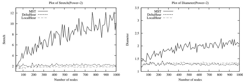
**Figure 8.** Plot of stretch and diameter for the MST and DeltaHeur scheme with random link costs.
