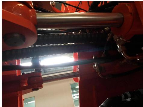
Figure 5. Steering mechanism of a FW50GL loader.
